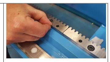
5. Place the second section of rack and approach the screws without tightening them
