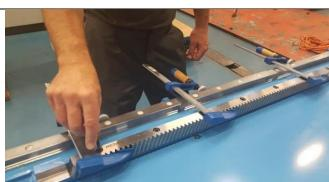
3. Tighten the screws to the tightening torque shown below
