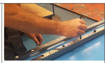
2. Press the rack against the frame with a clamping tool
