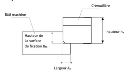
The minimum fixing surface height Bfh depends on the rack height ha and the selected module m.
