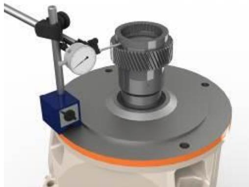
Shaft radial run-out measurement
