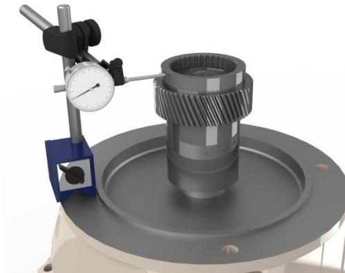
Shaft radial run-out measurement
