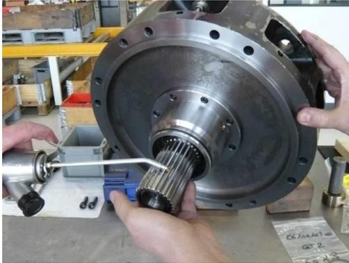
6. Apply grease on the central lip seal. Grease used must be compatible with gearbox oil lubrication.
