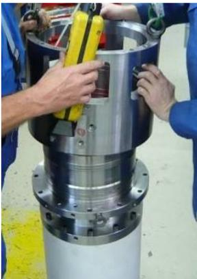
6. Fix the water jacket with screws.
