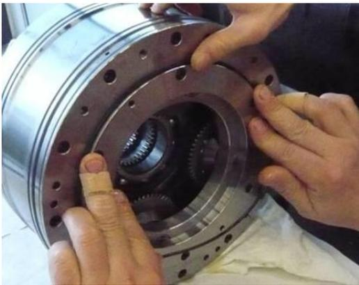
5. Use the tool 2, previously heated at 100°C, to heat the inner race of the gearbox central bearing (minimum 3 minutes).
