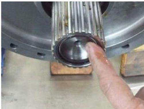
7. Check that the slide dog is in "direct ratio" position
