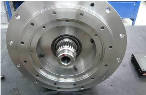
4. Grease all external surfaces of the motor shaft (use KLUBERPASTE 46 MR 401 or FAG Montage paste ARCANOL).
