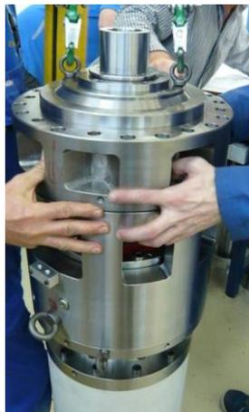
9. While bringing the spindle onto the gearbox and motor, oscillate the spindle shaft to find a proper teeth orientation for the introduction of the spindle shaft into the slide-dog.
