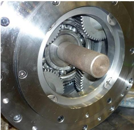
6. Mount the tool 1 into the slide dog and check the good rotation of the system.
