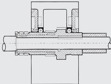
The accessory fitted to the reaction sleeve must be adjacent to the bearing to avoid excessive bending of the supporting shaft
